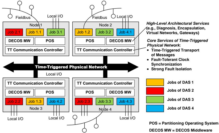
Fig. 1. Distributed System in the DECOS System Architecture
