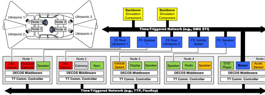
Fig. 5. Exemplary Integrated System with Environmental Simulation
