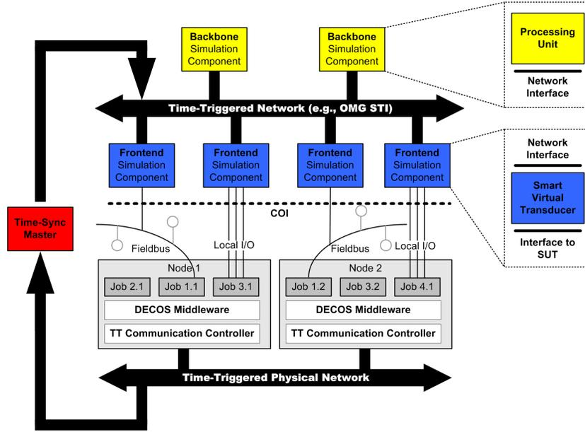
Fig. 2. HiL simulation with an Integrated System
